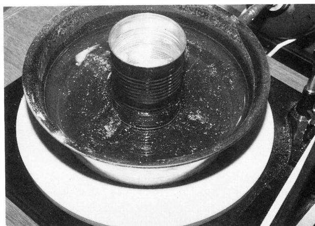
FIG. 6. The laboratory simulation of large-scale atmospheric motion following the work of Fultz et al. (1959).
