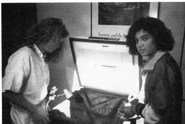
FIG. 5. One of the student lab teams forming ice crystals in a freezer chest by sprinkling shaved dry ice into the chest. (Kelly McNerney is on the left and Daphne Fontenot is on the right.)
