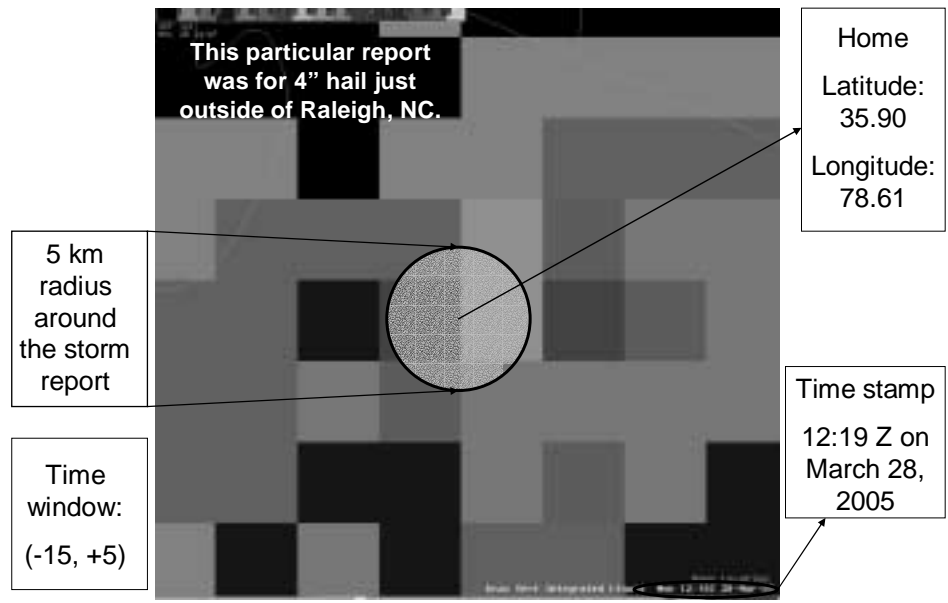
FIGURE 2. An illustration of several aspects of the event verification. By inserting the latitude and longitude, the cursor position stays in the exact spot of the report when recording all 17 products. Using the time stamp in the bottom right corner allows for watching the time window (-15, +5). The black circle around the “home” point signifies the 5 km radius. Features in AWIPS allow for the value of where the cursor is to display to the user, allowing for the value anywhere on the screen to be read and recorded. This particular report shows the 4 km VIL. It so happens that the maximum in the time window occurred in the same time frame as the actual and maximum radius product reading. The value for all three values recorded for 4 km VIL was 35 g/m 2 .
