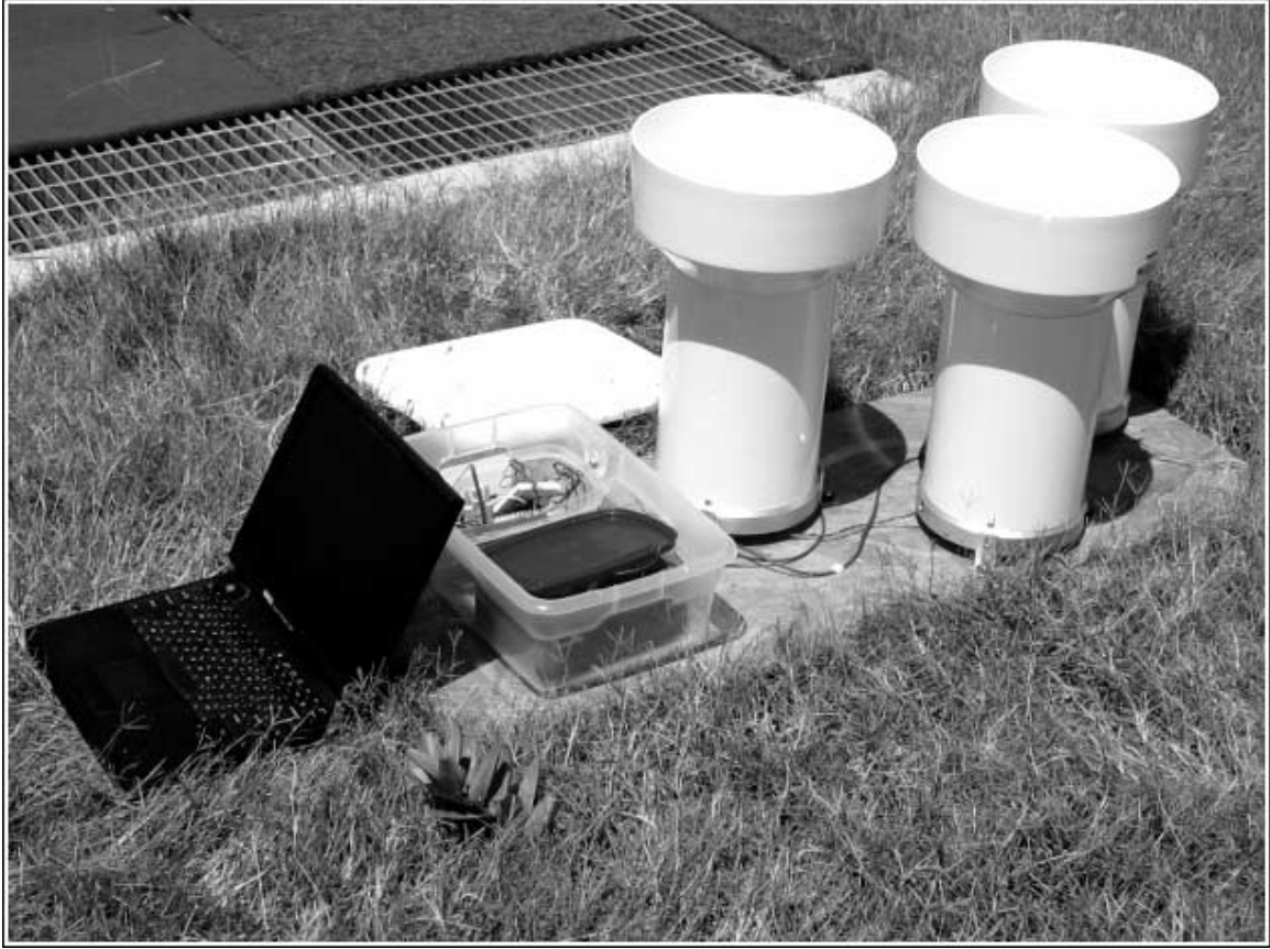
Figure 5. The PicoNet test site at NSSL, consisting of three rain gauges, 12V battery, CR200 datalogger, and the laptop used to extract the data.
