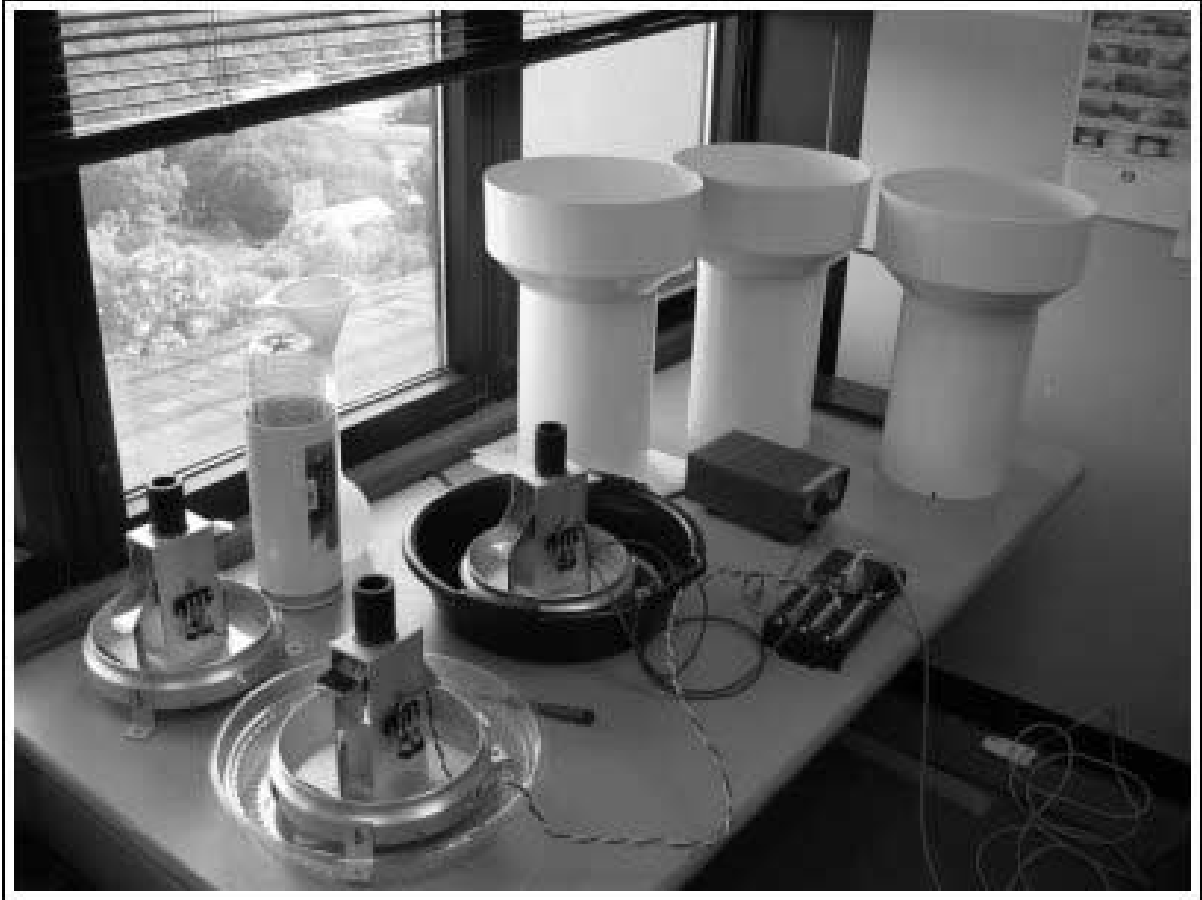
Figure 2. Display of the Mesonet calibration method used in accordance with the three gauges and CR1000 datalogger.
