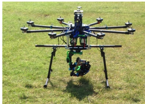
Figure 1: The UAV built by the ARRC for use in the calibration of the phased array radar.
