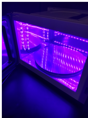
Fig. 2. Inside of the Microwave Oven as an UV Exposure Unit
