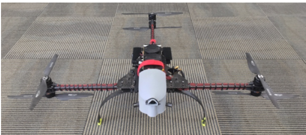
FIG. 6. Photo of the CopterSonde 3, the rotary-wing Y6 UAS utilized in this study to sample vertical profiles of O_3 .
